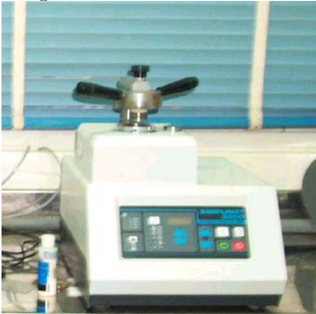
Fig 5: A Hot Mounting Press
