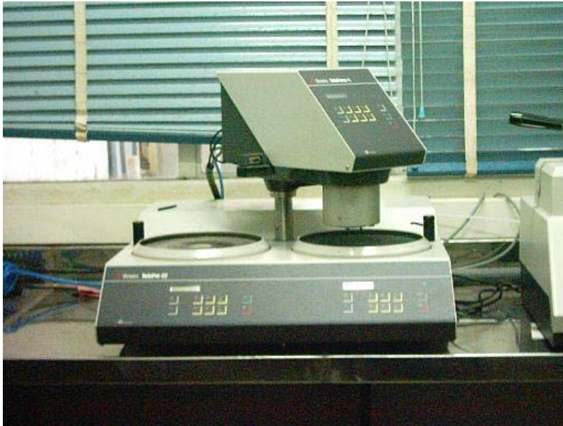
Fig 2 : An Automatic Polishing Machine with Two Rotating Discs
