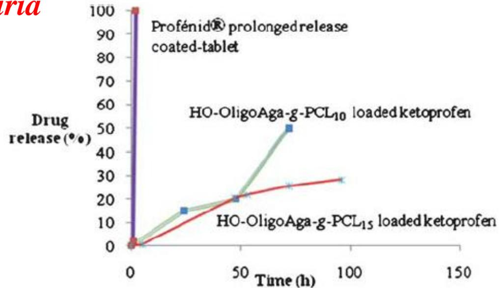
Fig. 5 Comparison of drug release profiles in PBS at 37 °C.
